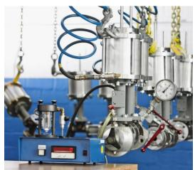
Furthermore each valve produced in KÜHME works is individually tested as per EN 12266-1 ensuring seat leakage class A. As leakage rate A as per EN 12266-1 allows no detectable leakage the performance is better as per comparable standard ANSI/FCI 70-2 and leakage class VI which still allows a certain leakage depending on the seat diameter. The same is highlighted in the comparison of both standards below:
